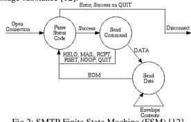
Fig 2: SMTP Finite State Machine (FSM) [12]
