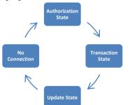
Fig 1: Post Office Protocol (POP3) Finite State Machine
