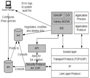
Fig 4: IPsec protocol suite - Internal structure [21]
